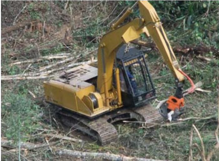
A single drum winch/grab combination prebunching for the Alpine Shovel Yarder.
